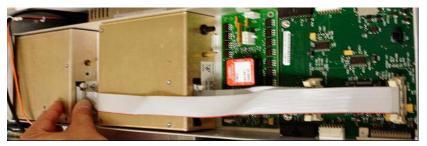
Figure 7 Connecting the APCI HV power supply to the valve PCA.
